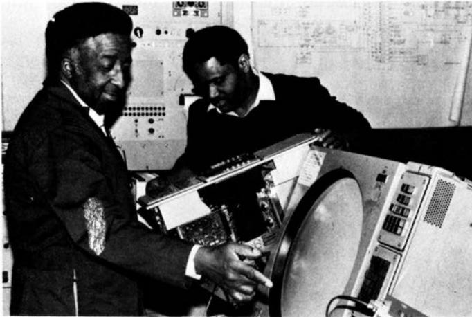
Electronics technicians Sam Graves (left) and Ed Taylor make final adjustments on one of the sector's 52 plan view displays.
