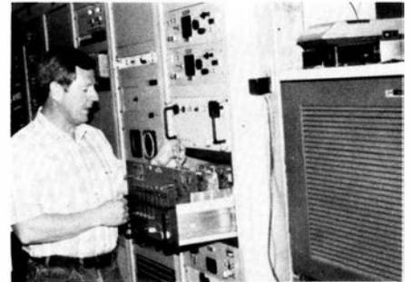
*At the Baton Rouge Sector Field Office, electronics technician Richard Stanton performs a check of the instrument landing system remote monitor.*
