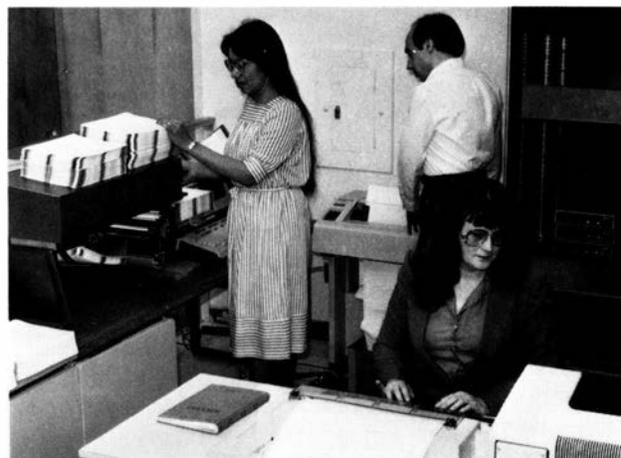
A CAMI team handles the 1984 survey. Lena Dobbins (left) loads the optical-mark scanner with surveys, while Lendell Nye checks the printer to ensure that the data is being read correctly onto magnetic tape. Carolyn Dollar enters commands into a terminal to permit scanned information to be transferred from the tape into the computer for analysis.
