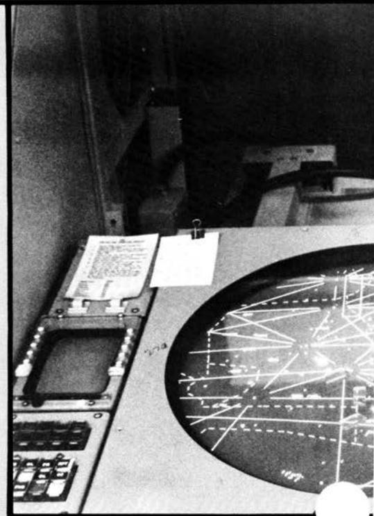
*An enhancement to the Third Generation ATC System with limited alphanumeric and shrimp board.*
