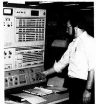
*Computer technician Robert Hirsch prepares to load a diagnostic program into the center's IBM 9020 computer.*
