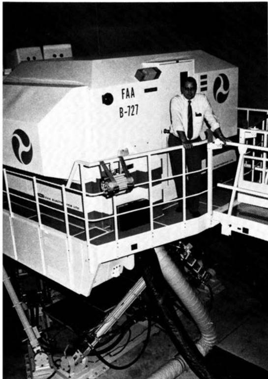
*The study is looking into the possibility of less-complex flight simulators than this Boeing 727 unit at the Aeronautical Center that will provide adequate training at less cost. Simulation supervisor Lester Groves stands on the catwalk.*
