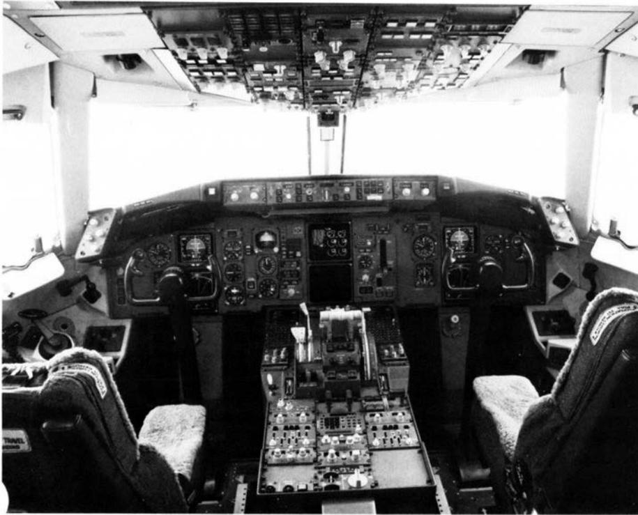
*The cockpit of a Boeing 767 reflects the state of the art in cockpit information transfer, showing six electronic displays in place of electro-mechanical ones, including, for example, CRT displays of artificial horizons.*
