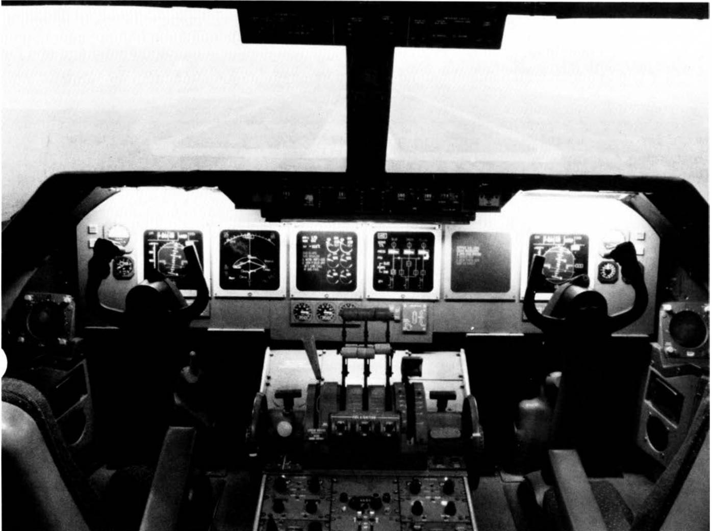
*This experimental cockpit panel by the National Aeronautics and Space Administration shows a wide array of cathode-ray tube displays and the use of color and symbols that may help pilots in discriminating among functions.*
