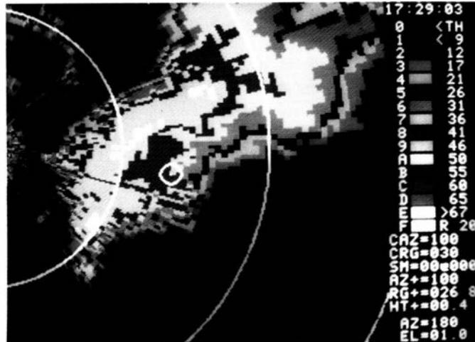
A segment of a Doppler radar display at the National Severe Storms Laboratory looking inside a weather front.
