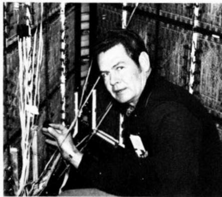
*Bob Hutchins, central computer complex technician in the Flight Data Processing Unit, attaches logic analyzer probes to the compute element 1 of the IBM 9020A.*
