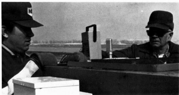
Electronics technicians Dale Engelhaupt (left) and Jack Schaeffer perform maintenance on the Chadron visual approach slope indicator (VASI).
