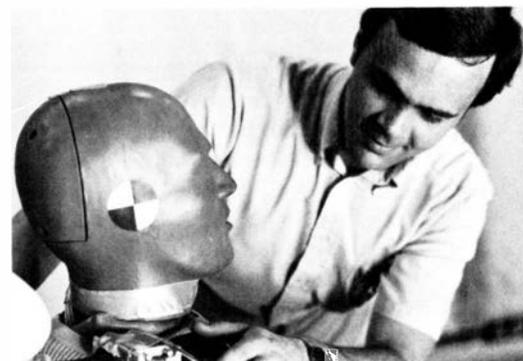
*To insure that all connections are secure for accurate readings, Van Gowdy, supervisor of the Biodynamics Research Unit, makes a final check of the test dummy.*
