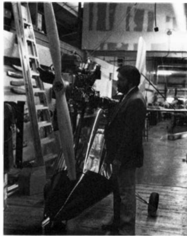
Following a static load test on a Pioneer ultralight, inspector Ness checks it over for deformation.
