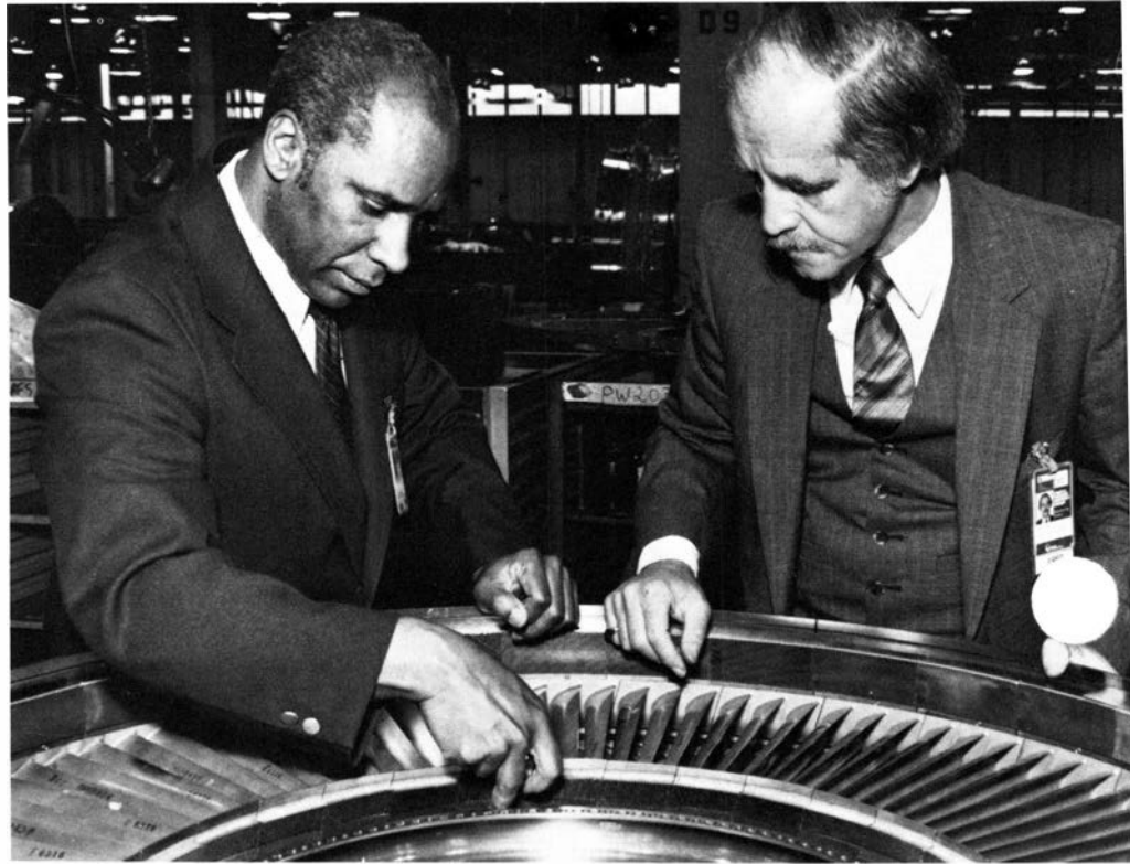
Al Pereira (left), manager of the Windsor Locks, Conn., Manufacturing Inspection District Office, reviews assembly techniques for a P&W 2037 engine's low-pressure turbine vane with Fred Polodori of Pratt & Whitney.
