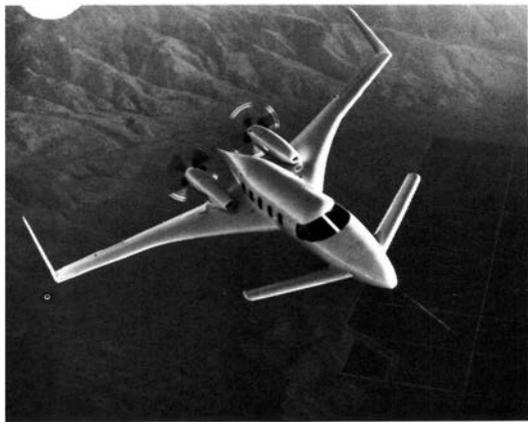
*Also a 400-mph pusher turboprop with a canard is Beechcraft's Starship 1, which also carries drag-reducing winglets.*
