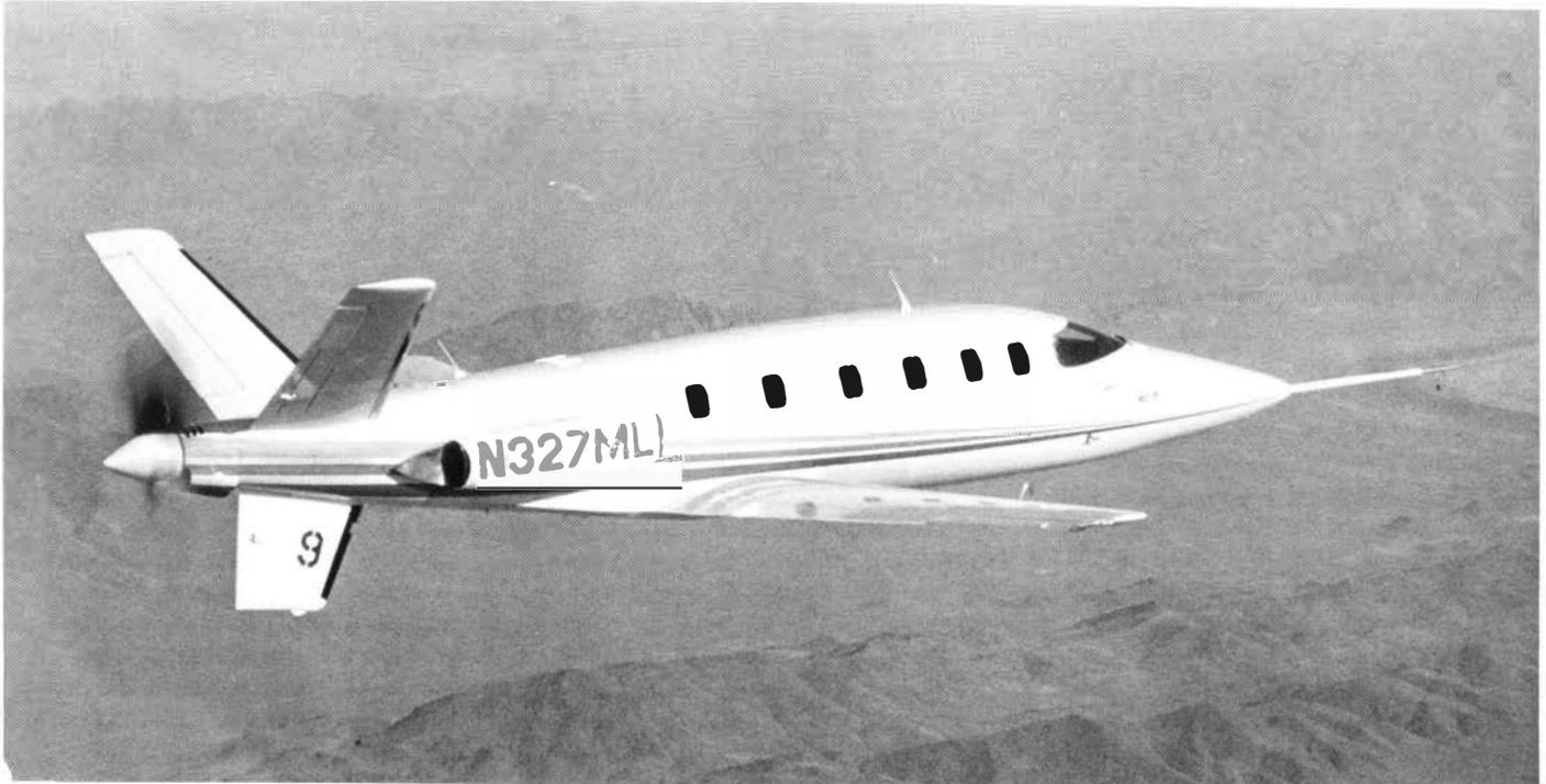
*This was the first production prototype of the Lear Fan, a graphite-epoxy-composite-skinned turboprop that has the prop separate from the jet nacelle.*
