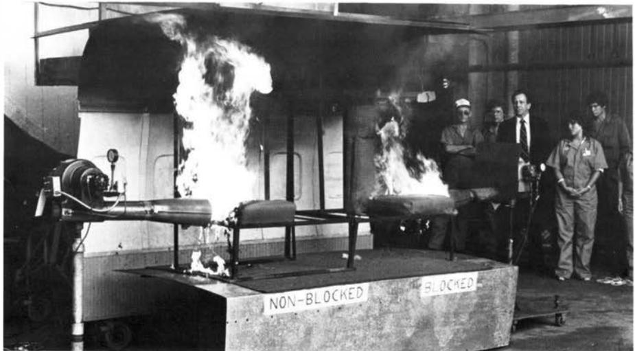
*In a demonstration of ongoing fire safety studies at the FAA Technical Center, an ordinary, non-blocked airliner seat and one incorporating a blocking layer around the foam cushions were set afire. The blocked seat took longer to ignite.*
