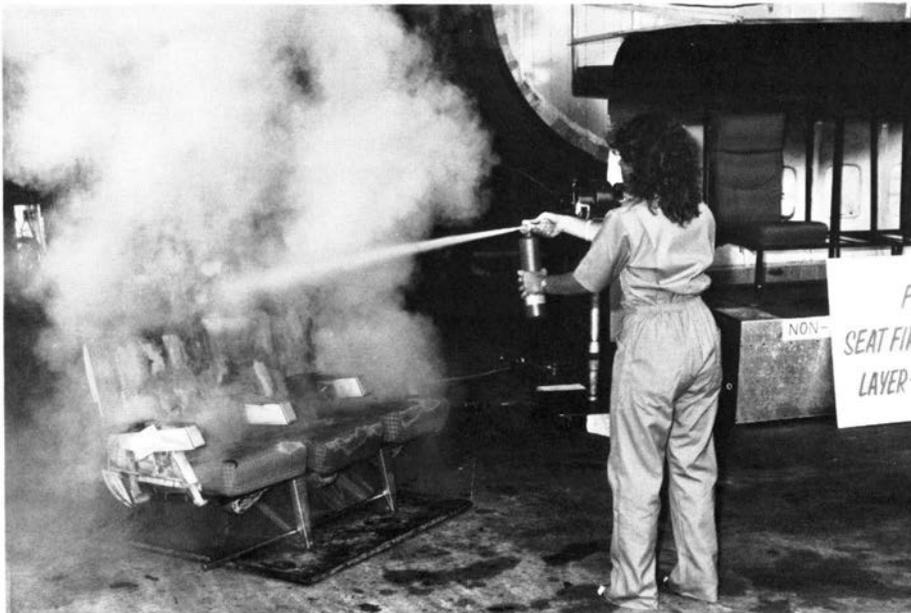
*A Tech Center employee extinguishes an airline seat fire with a new Halon 1211 extinguisher which does the job faster and at greater range than other types.*
