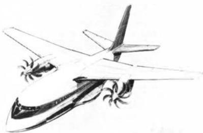
The thinner and shorter eight- to 10-blade, swept-tip propeller, or propfan, is expected to offer quieter, fuel-efficient operation at speeds comparable to those of jetliners.
