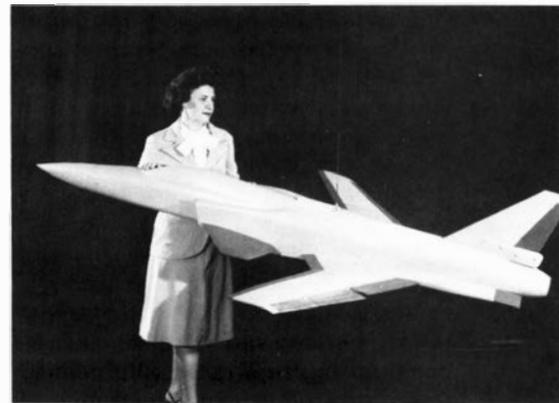
Langley aerospace engineer Sue Grafton holds a wind-tunnel model of a Grumman forward-swept-wing aircraft. This configuration permits the wingtips to remain unstalled at high angles of attack.
