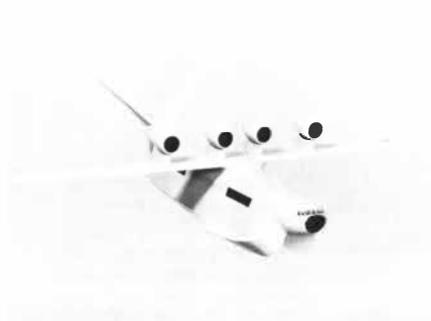
A blended-fuselage catamaran is a feature of this Lockheed-Georgia amphibian, which could carry a 63-ton payload. It could fly 3,200 nautical miles and, with its wing 26 feet above the waterline, could sit in a sea state 6 (20-foot waves). Hydroski assists takeoffs and landings.
