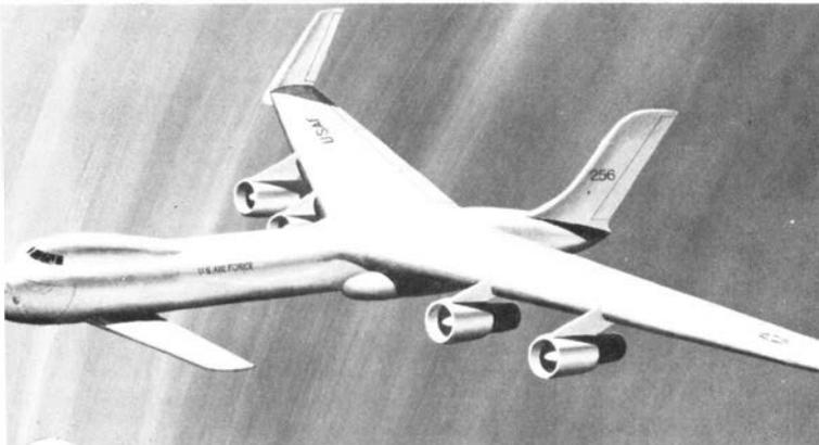
This configuration is for a global-range nuclear-powered argoliner for payloads of 200 tons. It would use supercritical airfoils, a free-floating canard with spanwise blowing for horizontal control and high-bypass-ratio engines.
