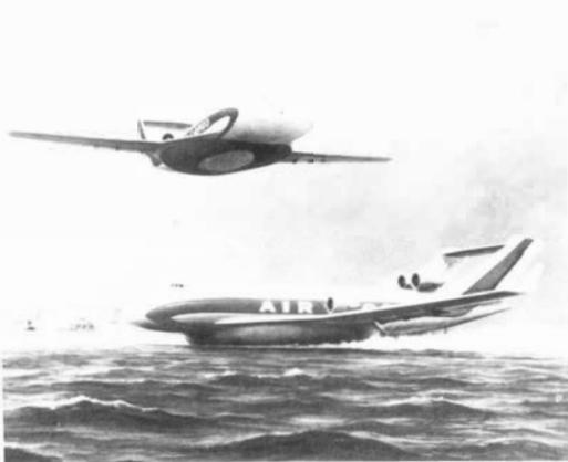
One NASA answer to the constraints of airport size and the need for larger cargo aircraft is the air-cushion landing gear airfreighter, which could use runways, water and even unprepared sites. Bell Aerospace Textron has studied it.
