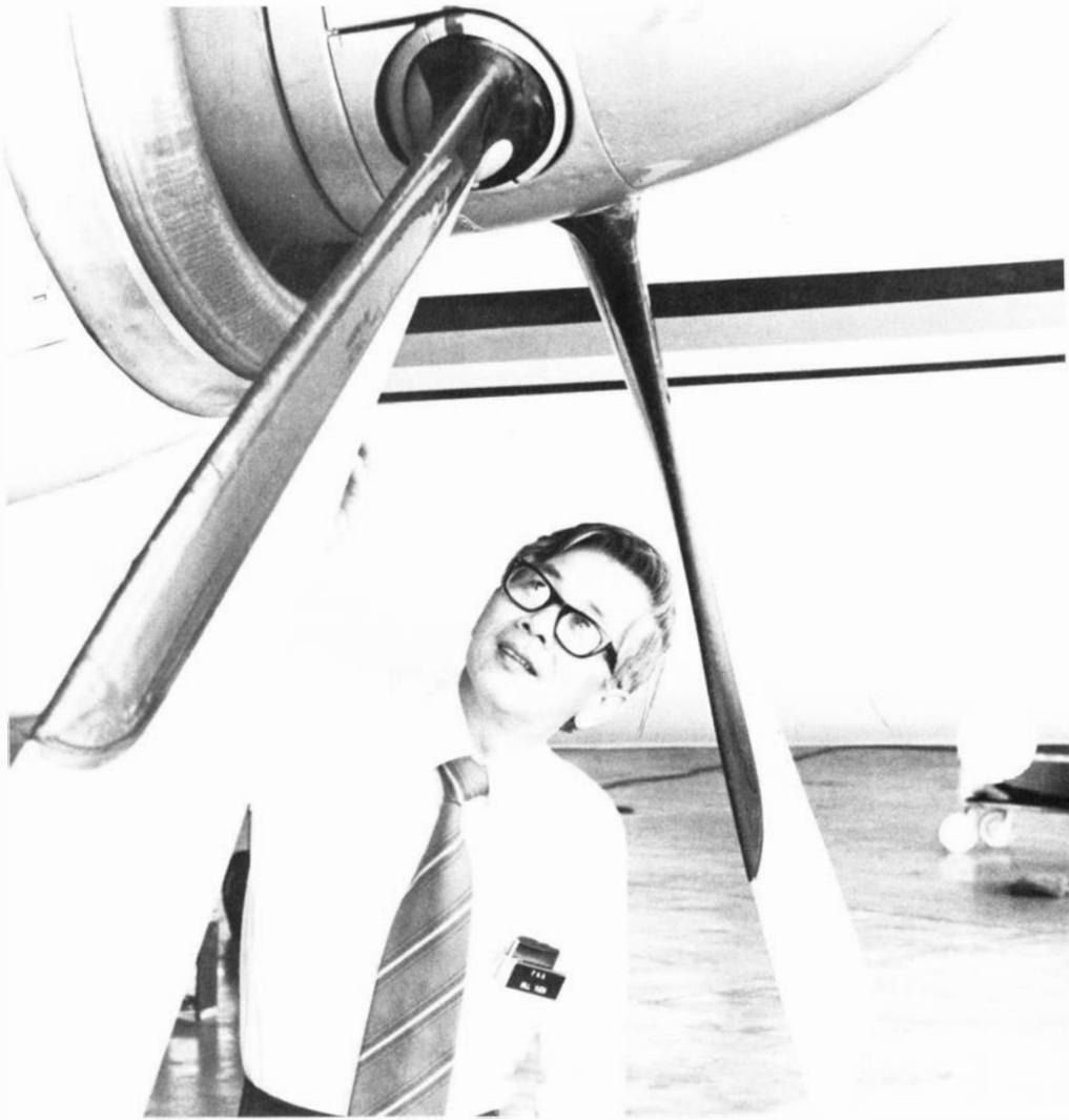
Aviation safety inspector Bill Yuen checks the surfaces of a propeller on a transport-category aircraft.
