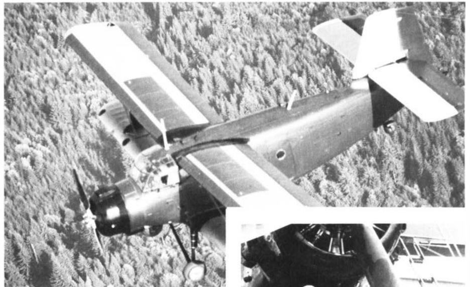
aluminum, it's 7,276 pounds empty and over 11,000 pounds at gross, holding two in the cockpit and 14 passenger seats. It cruises at 124 mph; top speed is 161; its range 560 miles; and its ceiling 16,400 feet. It has a Shetsov air-cooled radial engine that develops 1,000 hp, driving a four-blade, variable-pitch, constant-speed propeller.
