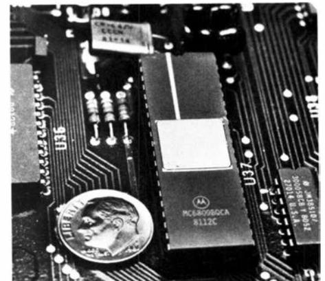
A microprocessor integrated-circuit module containing a large silicon chip is compared to the size of a dime. The circuitry in the chip is perhaps equivalent to that found in about 50 TV sets.
