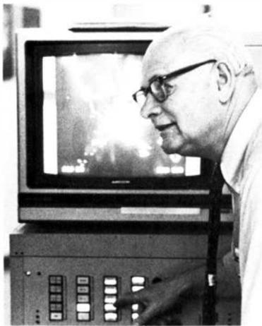
Bud Lacey, National Weather Service meteorologist at Washington headquarters' Central Flow Weather Support Unit in the Systems Command Center, demonstrates the depiction of various precipitation intensities on the facility's new color weather radar display.
