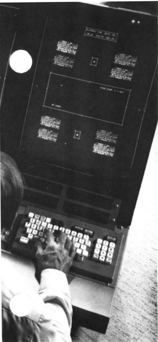
ETABS (Electronic Tabular Display Subsystem) is being delivered by Sanders Associates, Nashua, N.H., to the Tech Center to be used as an engineering model. ETABS functions for flight data display and infrared touch entry will be integrated into the ATC sector suite.
