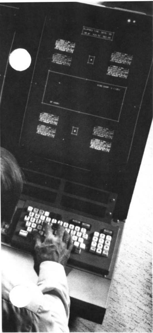
ETABS (Electronic Tabular Display Subsystem) is being delivered by Sanders Associates, Nashua, N.H., to the Tech Center to be used as an engineering model. ETABS functions for flight data display and infrared touch entry will be integrated into the ATC sector suite.
