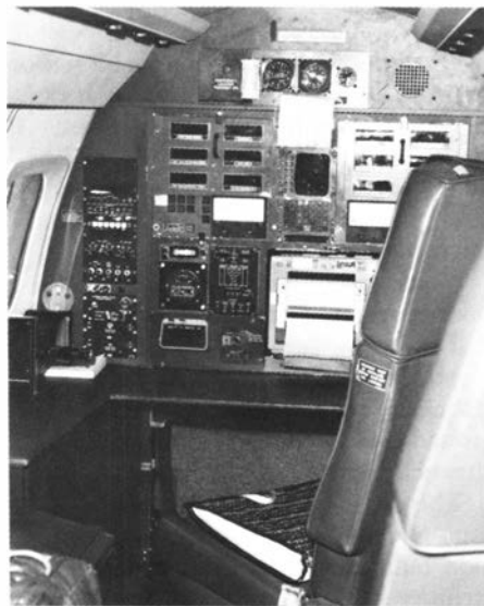
Improvements to flight inspection include the Automated Flight Inspection Computer System, now installed in 15 Sabreliner 80s and five Jet Commanders.
