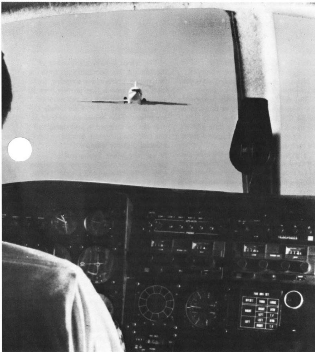
Two FAA Technical Center aircraft—a B-727 and a Convair 580—really fly at each other deliberately to trigger collision-avoidance equipment installed in their cockpit panels.
