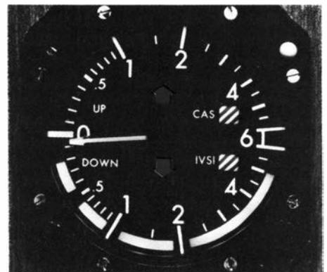
Another display to be found in a TCAS II-equipped plane is a modified instantaneous vertical speed indicator (IVSI), here indicating the resolution advisory "do not descend" by means of the lighted bars. The pilot must keep the IVSI pointer out of the descent rates covered by the illuminated segments. An alternate climb or descend advisory could be displayed by lighting the appropriate arrow in the center of the instrument.
