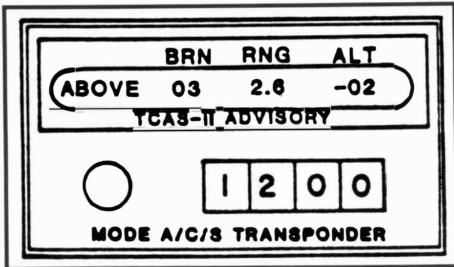
The TCAS I transponder will display bearing, range and altitude information from intruding TCAS II-equipped aircraft.
