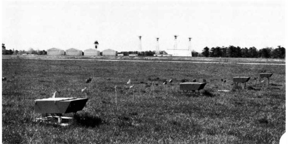
Four PAPI units are lined up at Teterboro, N.J., Airport to test the British glideslope system in a general aviation environment.
