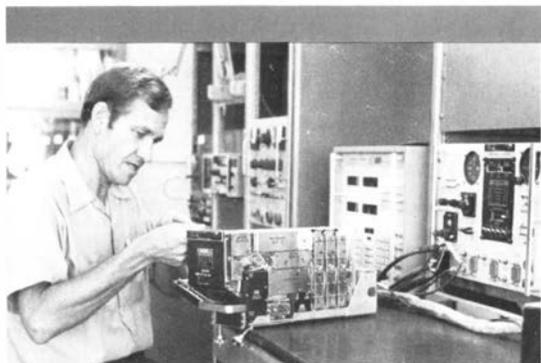
Electronics technician Ted Whitman works on a weather radar unit for a Sabreliner in the Minneapolis FIFO's own maintenance shop.
