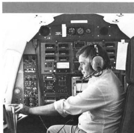
Electronics technician Don Stokes' office during a flight check is a compact, computerized array of avionics at the rear of a Sabreliner flight-inspection plane.
