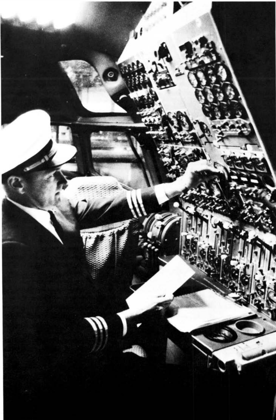
By 1961, the flight engineers handled instrument monitoring not servicing functions, such as this one aboard a DC-8.
