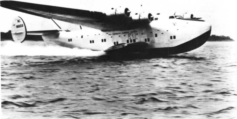
Pan American's Yankee Clipper carried a mechanic in the 1930s who could actually service the plane's engines in flight.
