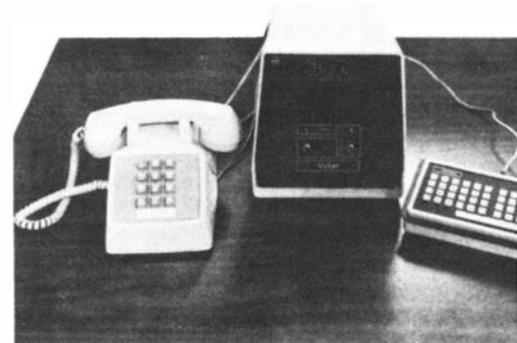
A VuSet CRT acoustically coupled to a push-button telephone will be able to retrieve alphanumeric data from the FSS computers, as well as display a digital map weather radar summary, such as the one shown at the top for the Houston, Tex., area.
