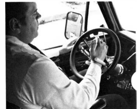
His throttle is a motorcycle-type control at his left hand; three pegs on the steering wheel support his weakened hand for spinning it.
