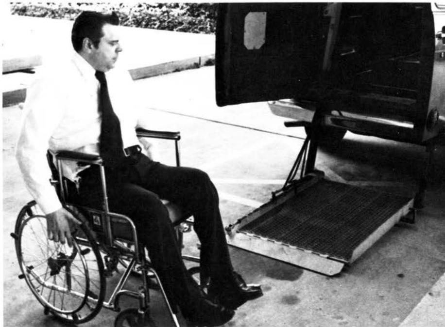
He enters the van facing forward but turns around to leave to assure himself that the platform is fully lowered. The control panel for the lift and doors is on the left door.
