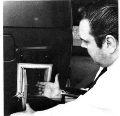
Hawkins' solo performance with the Blue Max starts with a toggle switch panel on the rear fender, which opens the doors and lowers the lift gate.
