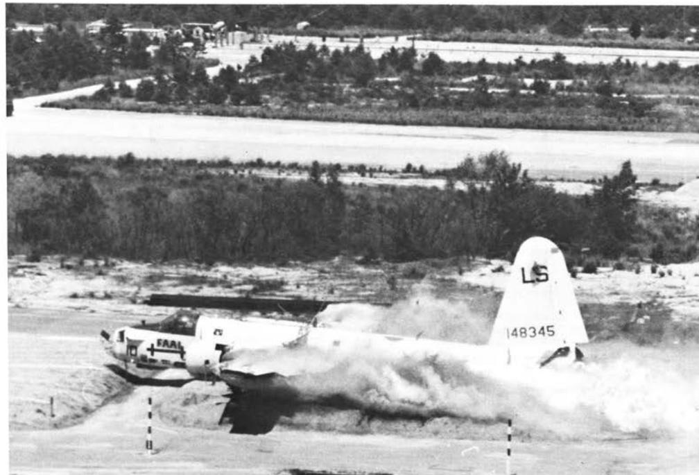
In a test at Lakehurst, N.J., when a transport-category aircraft loaded with regular jet fuel was hurtled along a catapult into a mound of earth and fuel was spilled and ignited, the plane was engulfed in a ball of flame.
