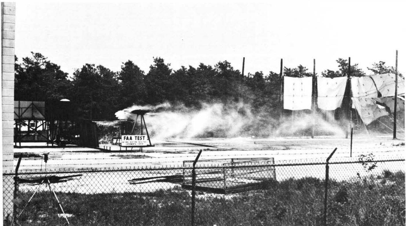
Standard aviation fuel spilled from a wing section and ignited at the FAA Technical Center's Wing Spillage Test Facility goes up in a huge fireball. (top)
