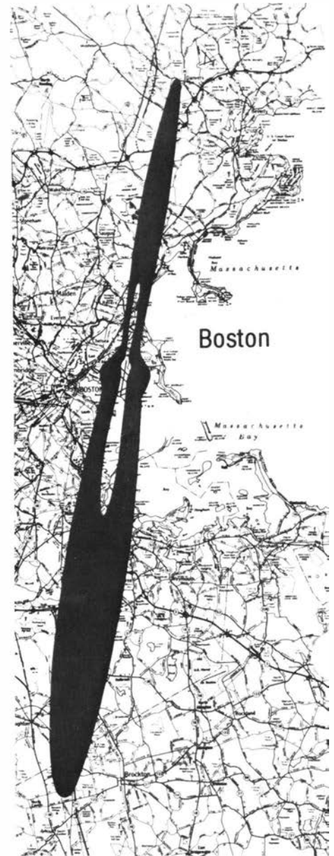
The noise "footprint" of a DC-8 over Boston. The area exposed to 90EPNdB (effective perceived noise decibels) with its earlier engine (black outline) is contrasted with the area affected by the plane with a new, quieter engine installed in response to the FAR (white outline).
