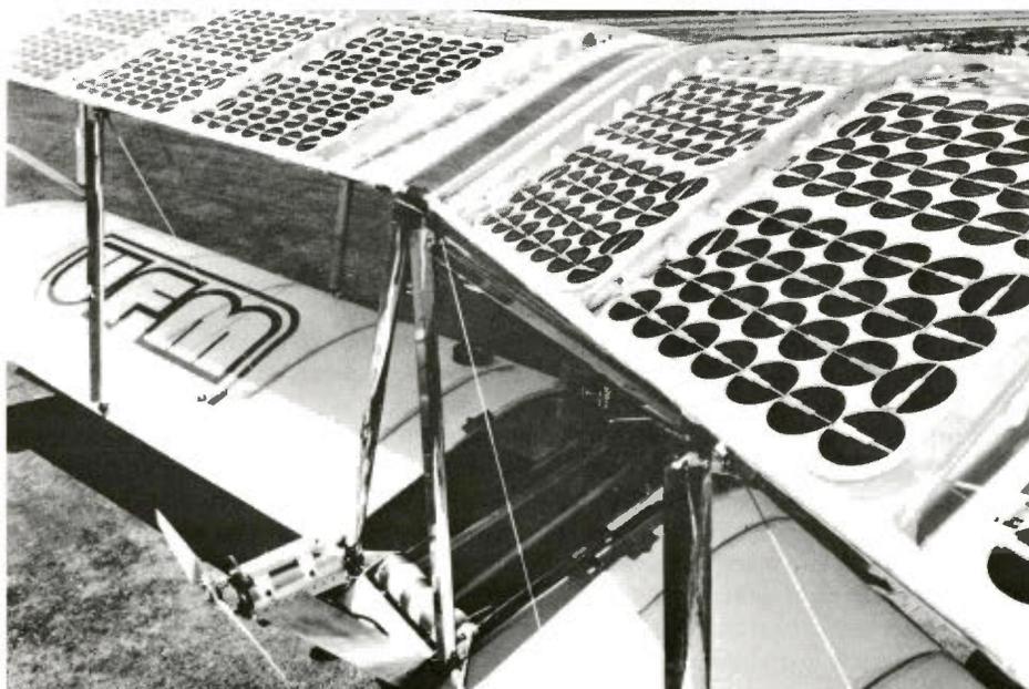
Larry Mauro demonstrated his Solar Riser—the first solar-powered aircraft—at the Experimental Aircraft Association's annual fly-in at Oshkosh, Wis., last summer. The upper wing is arrayed with 600 photovoltaic cells that power a 4-hp electric motor . . . briefly. (Ultralight Flying Machines photo)
