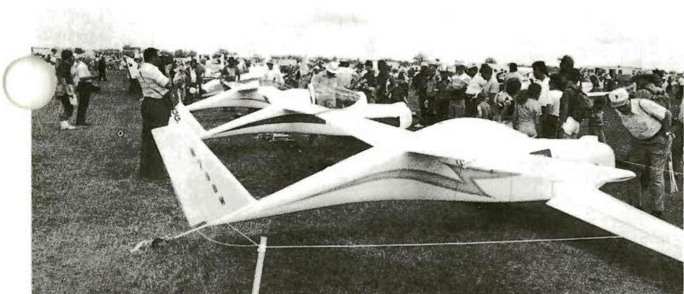
The Quickie is an unusual canard design: The wide-spreading wheel struts carry the elevators. Its 18-hp engine pulls it an average 110 mph at a miserly 65 miles per gallon.
