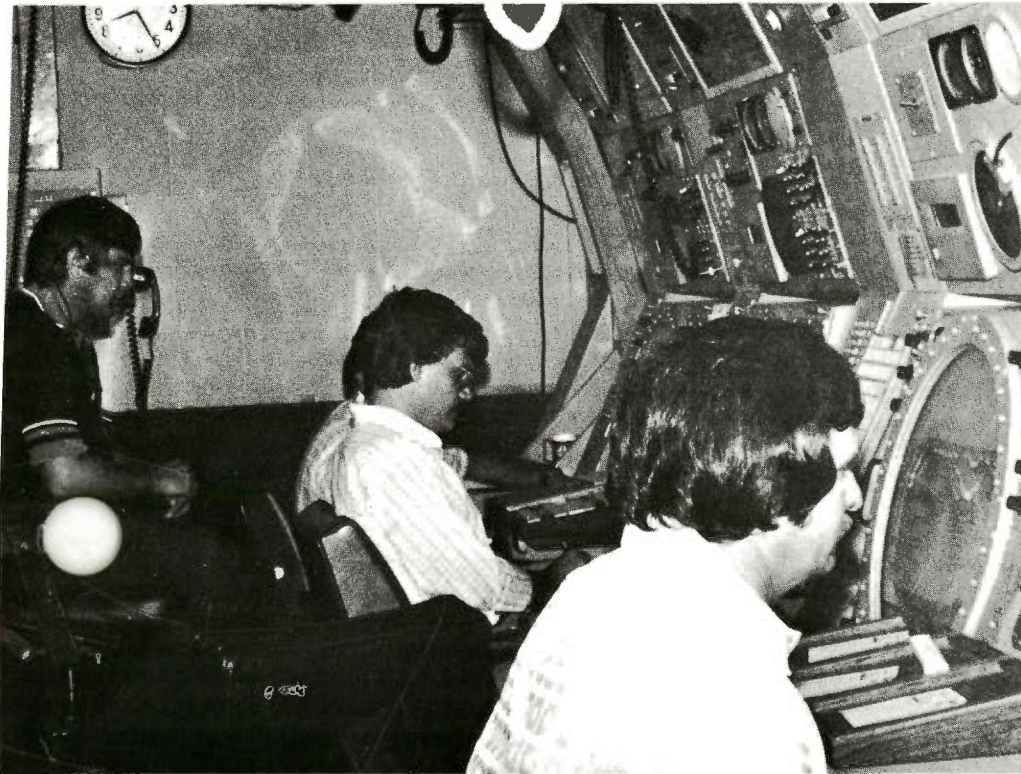
One might say that ATCSs Scott Craig, Bob Gore and Hal Wise (left to right) get less eye strain in the West Palm Beach, Fla., TRACON, now that they have the 22-inch ARTS II scopes in place of the nine-inch TPX-42s. The real improvement is in having aircraft identity and altitude data tags.
