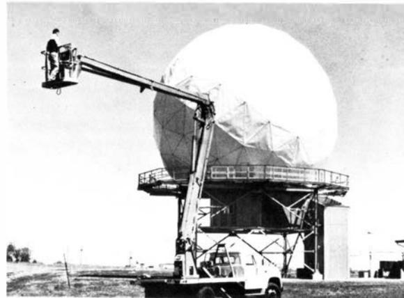
*Measuring the field-density strength of a new ARSR-3 from a cherry-picker is Gerald Markey, chief of the Frequency Engineering Branch of the Airway Systems Division, Airway Facilities Service. The measurements are taken on the main beam axis heading toward the antenna until a 10 mw/cm<sup>2</sup> reading is reached—the safe-exposure limit.*
