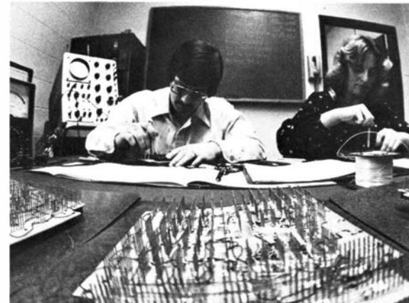
*Dave Euler, developmental engineer, and Candy Dobkins, electronics technician trainee, assemble re-enforced-rate computers, which consist of integrated-circuit boards and a forest of pins and wires.*
