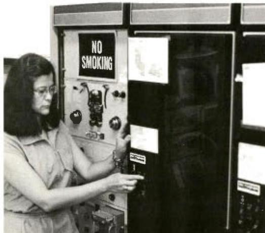
*Dr. Carol Roberts of the National Transportation Safety Board switches on a computer that provides readouts from a crashed aircraft's digital flight-data recorder.*
