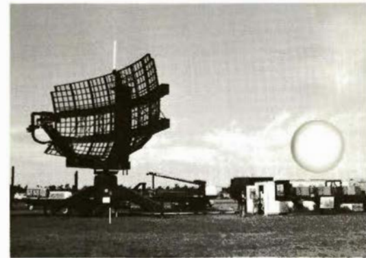
Four mobile ARSR-3s are being supplied for emergency backup under the Westinghouse contract. The antenna is assembled from three sections and operates from a flat-bed truck with bracing legs on the ground. It's supported by a power-plant trailer and an electronics trailer.
