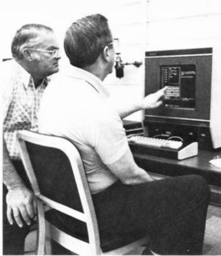
*In the FAA Academy's Flight Standards Airspace and Procedures Section, instructor Joe Reddin (left) monitors the use of a Plato V display under evaluation, which duplicates the RNAV computer in flight inspection airplanes. Battle Creek, Mich., FIFO pilot Leo Blakely punches the buttons.*
