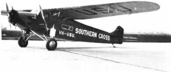
The Pacific-hopping Southern Cross carried wing tanks and a tank under the pilot's seat in addition to the main tank, for a total of 1,298 gallons of fuel.
