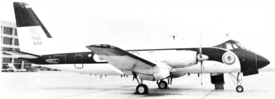
*Flying in support of the center's collision avoidance system (CAS) tests is N-48, one of two Gulfstream 1s. It is also used for RNAV research and is equipped with avionics for CAT II flight for runway-lighting.*
