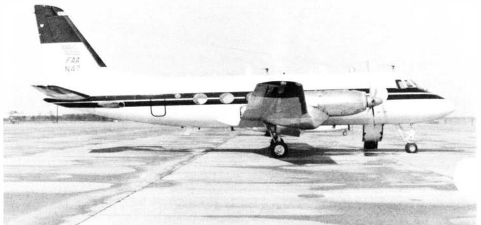
*The Convair 580 turboprop—N-49—is also instrumented for use in the development of CAS and has CAT II capability for the runway-lighting programs. It also sees service for Omega and Loran-C testing.*
