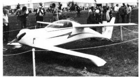
The unusual Rutan Quickie made its first appearance at this year's show. Depending on how you look at it, its ailerons or its elevators are in the wheel struts. It's claimed to have traveled from California on \$25 worth of gasoline at 127 mph.
