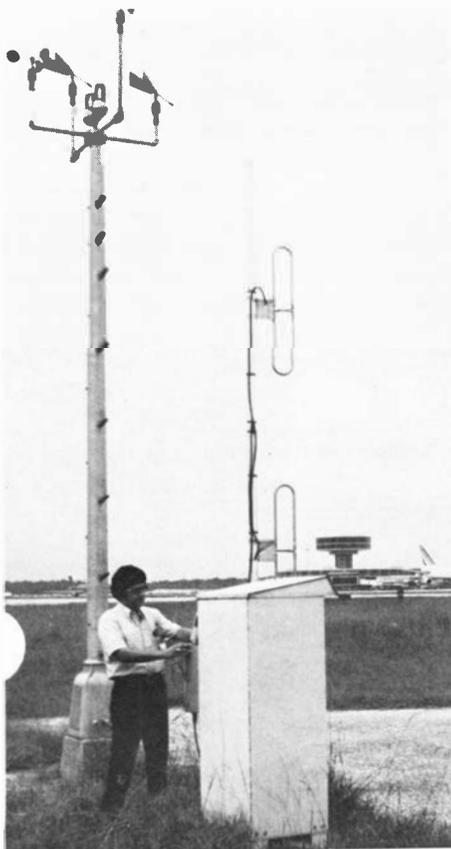
Electronics technician Arthur Zepeda of the Houston Intercontinental Airport Sector inspects the centerfield anemometer and its sending unit, which is part of the Low-Level Wind-Shear Alert System being tested there.
