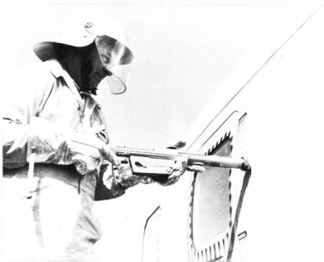
**FIRE-FIGHTER**—No, it's not a rebel soldier from Princess Leia's starship! It's Chuck Urban, NAFEC aerospace engineering technician, testing an aircraft-skin penetrator nozzle developed by the USAF for injecting extinguishing agents to combat fires inside aircraft.
