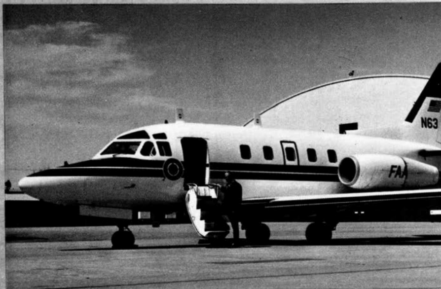
ANOTHER ONCEOVER —The Sabreliner that Western Region Director Stanton took delivery on arrived at the Aeronautical Center for avionics fitting out and service for flight inspection. Dale Crawford, chief of FINFO, looks through this last of the Sabreliners entering the agency's fleet.
