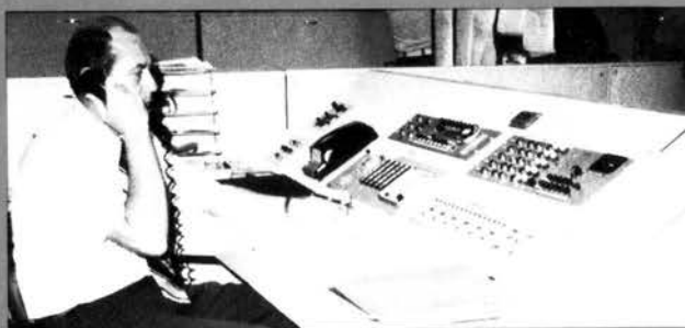
JUST A MOMENT, PLEASE —At the new Portland FSS in Hillsboro, Ore., assistant chief Bob Hogan handles a call over a new FAA-leased integrated voice communications system. Instead of keying for briefings, ATC interphone, intercom, emergency and airport direct lines, the specialist gets immediate handling of ATC interphone lines with automatic distribution in proper sequence of incoming briefing calls or automatic storage of them if the briefers are busy. He also receives visual and audible signals of all time-critical calls.
