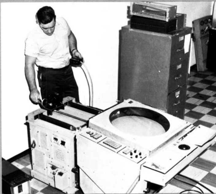
PROBLEM SOLVER —When the alphanumeric on an ARTCC scope go out, controllers have to tug the 325-pound scope into a horizontal position for the shrimp boats. Herman Regal, NAFEC modelmaker, along with Bill Einbinder and Irving Mower, devised a safe and inexpensive motorized drive to raise and lower the equipment. If the motor is inoperative, a hand crank is provided. Cost of the fix: less than $100.
