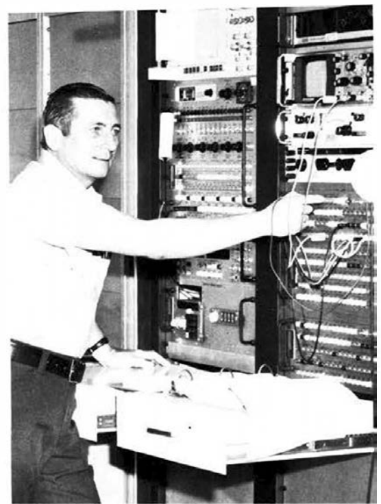
Avionics technician Nathan Parsons checks the alignment features of the Aircraft Services Base inertial navigation system maintenance equipment. The base's INS-RNAV repair station is the only one of its kind in aviation.
