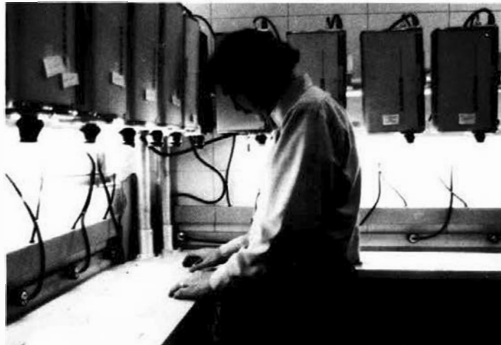
Teletypewriter operator John Rupp arranges weather reports and weather maps under a battery of closed-circuit TV cameras at the Phoenix, Ariz., FSS, saving the specialists time, effort and money in providing briefings via CRT at each position.
