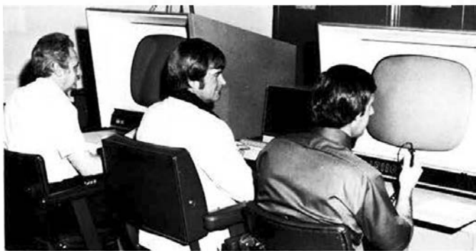
Three controllers in the oceanic ATC lab talk to an airplane thousands of miles away, using line-of-sight communications relayed through a satellite. The position of the plane—out of radar range—is relayed via data link and displayed.
