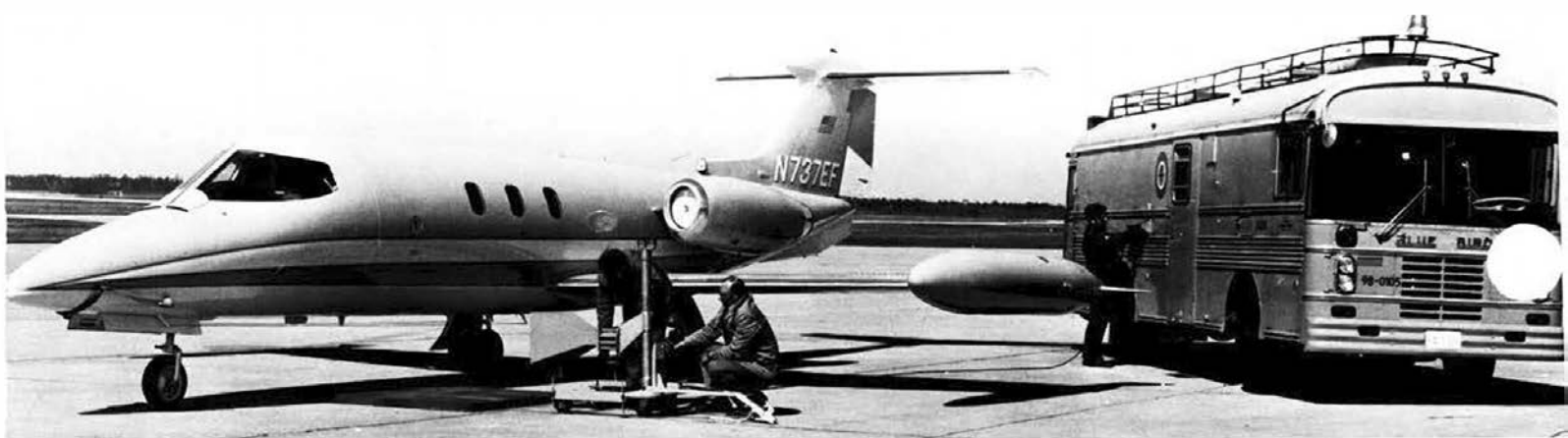
Technicians aim a horn antenna at a plane's beacon antenna in a test using a system housed in the van to check out transponder performance. It was demonstrated for the first time at the Reading Air Show in 1975.
