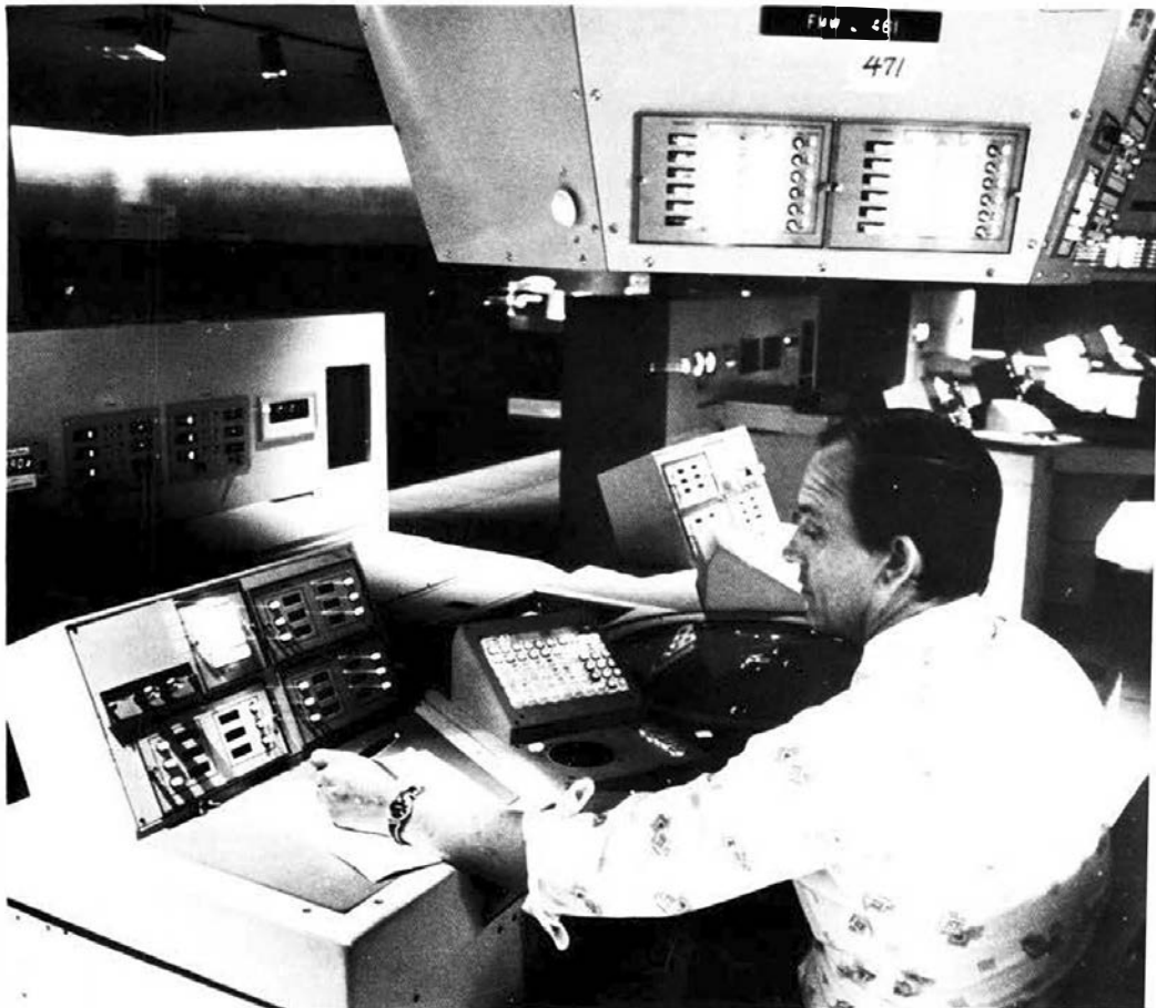
Concurrent with the commissioning of the last ARTS III of the originally programmed 64, Dallas-Fort Worth commissioned the Terminal Communications Switching System (TCSS), an automated network providing almost instant flexibility in position configuration. Controller Bill Ackley works the horizontal ARTS display, with TCSS lighted displays overhead and to the left.
