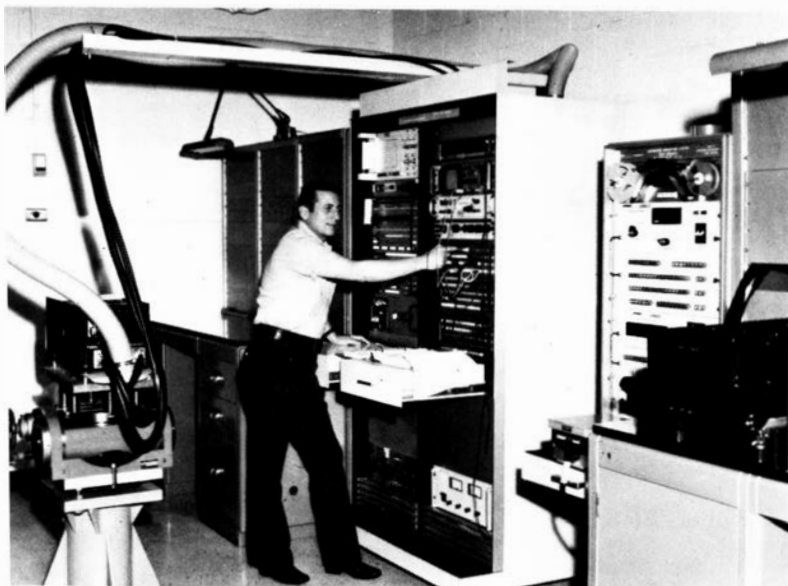
Nathan Parsons, avionics technician at the Aircraft Services Base, checks the alignment features of the new Inertial Navigation System maintenance equipment.
