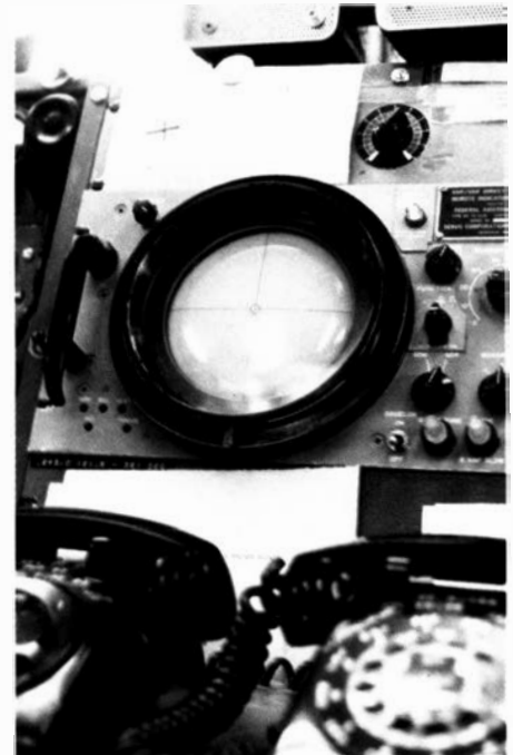
Pilots' lives depend on this small circular scope — Martinsburg's radio direction-finding console, which is effective to 100 miles, but usually gets closer work. The DF antenna is on the opposite page.
