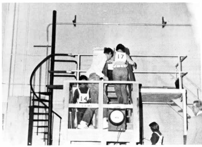
DOWN THE UP STAIRCASE —Going nowhere fast are some 30 individuals simulating a typical air-carrier passenger mix moving between decks and evacuating the upper deck of a wide-body aircraft. The Aeronautical Center study, involving the Depot, Flight Standards and CAMI, used a narrow passageway and straight and spiral staircases. Oscar Ball of Flight Standards is the project officer.
