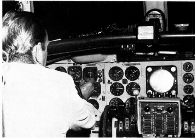
NAFEC test pilot John Ryan adjusts his ILS-VOR cross-pointer display that can be switched for MLS or ILS.
