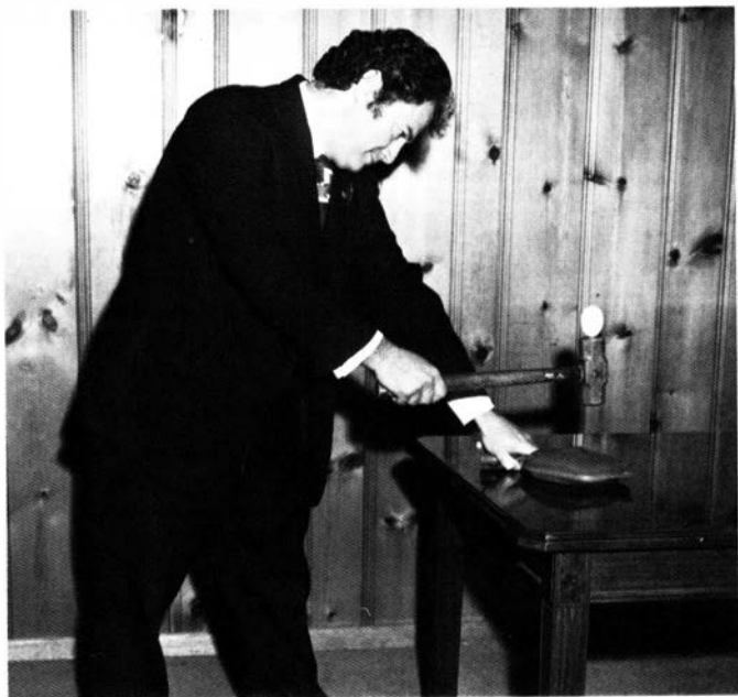
GENTLY, NOW — With an egg glued to a hammer, Bruce Rosenberg, NAFEC human factors psychologist, hammers on a rubber bag filled with an impact-absorber he invented that would make it useful for seat cushions, auto bumpers, etc.
