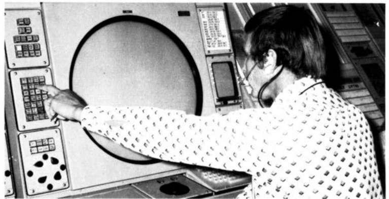
Though no radar image is apparent to the camera's eye, it is to controller Walter Schade, who asks the computer for additional radar information to be displayed.
