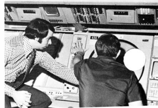
EPDS Don Schmidt instructs a controller on the modified ARTS III computer system that has been installed in the Anchorage ARTCC for processing and displaying digital data from the Murphy Dome long-range radar.
