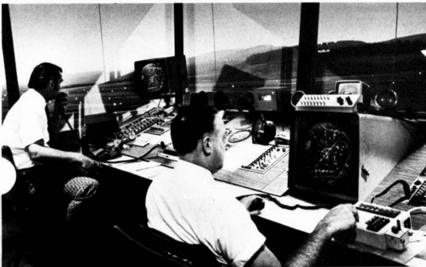
In tests of a prototype ARTS II system in 1973, controllers at the Wilkes-Barre/Scranton Airport received aircraft identity and altitude on their scopes.
