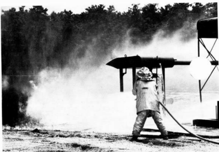
In an attempt by the Aircraft & Airports Safety Division to find the right thickened fuel that will not burn under certain conditions, firefighter Norman Irons uses liquid foam.
