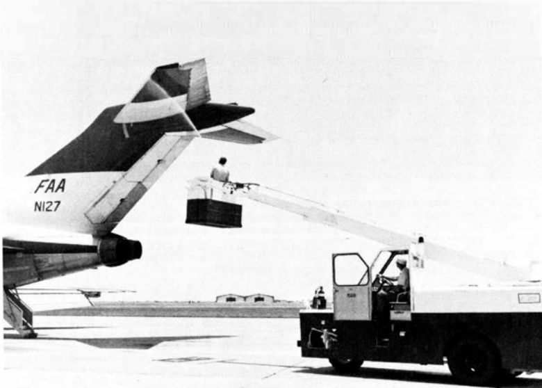
New at the Aircraft Services Base is this truck-mounted 42-foot boom with two-man basket designed for washing and de-icing aircraft. It has 1,000-gallon heated tanks for solutions, ground level hose reel and spray gun, pumping systems and cab-to-basket communications system.
