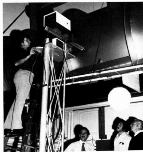
Technical photographer Joe Cox sets up an optical system to photograph fuel breakup in a wind tunnel. Observing (left to right) are Dr-Costos Polymeropoulos of Rutgers U. and NAFEC's Jim Valleley and Sam Zinn. They are investigating anti-misting characteristics of two jet fuels.
