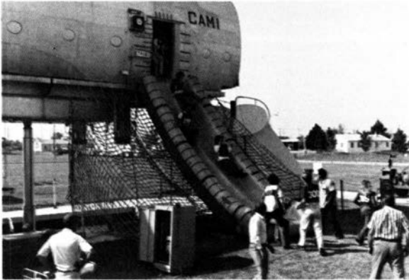
One of last year's projects for the Civil Aeromedical Institute (CAMI) was testing the rapid evacuation of the handicapped from a downed airliner using its evacuation simulator, which can be raised to 20 feet and can be tilted hydraulically about 15 degrees.
