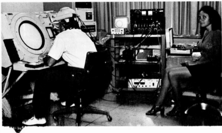
Color for radar scopes was evaluated as a method of reducing clutter, to code maps and alphanumeric tags and to check the readability of target data in varied color combinations. Paul Quick looks over one of the displays.
