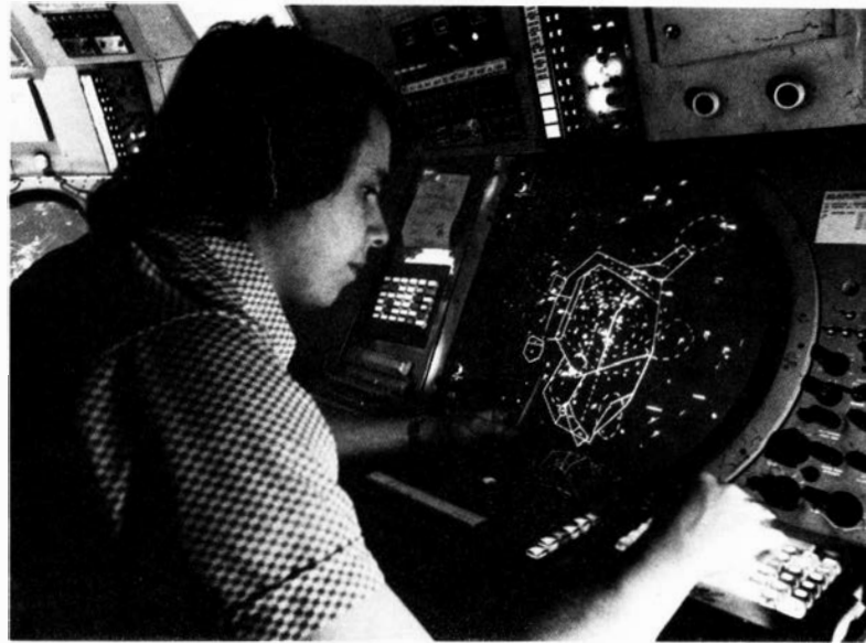
At his position before an ARTS III scope in the TRACON at Washington National Airport, Rico Imundo controls aircraft approaching Andrews Air Force Base in Maryland.
