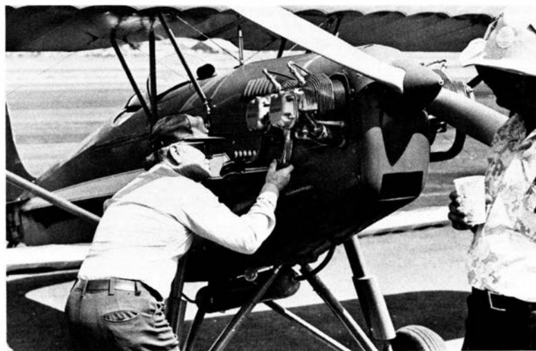
Accident prevention begins with a safe plane. At a September air show at San Diego's Gillespie Field, airworthiness inspector Jim "X-ray" Denniston of the San Diego FSDO checked the exhaust system of a Rose "Parakeet."
