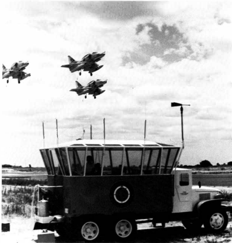
Navy A4Es drop their hooks and gear and come into Merced Municipal Airport, Calif., in an exercise supported by an FAA truck-mounted mobile control tower.
