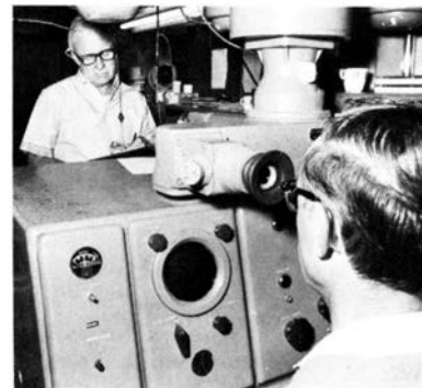
Dewitt Vernelson (left), Aeronautical Center, records data, as Charles Knapcik, O'Hare Airway Facilities Sector, monitors an APTAR scope that tracks aircraft for studying noise.
