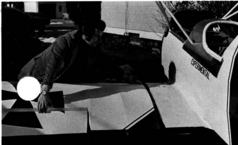
Perhaps he didn't have time to change out of his home-tailored sports jacket before getting to work on his home-built scaled-down Buecker-Jungmeister aerobat. Here, Lampton fits the lower wing into slots on the plane.
