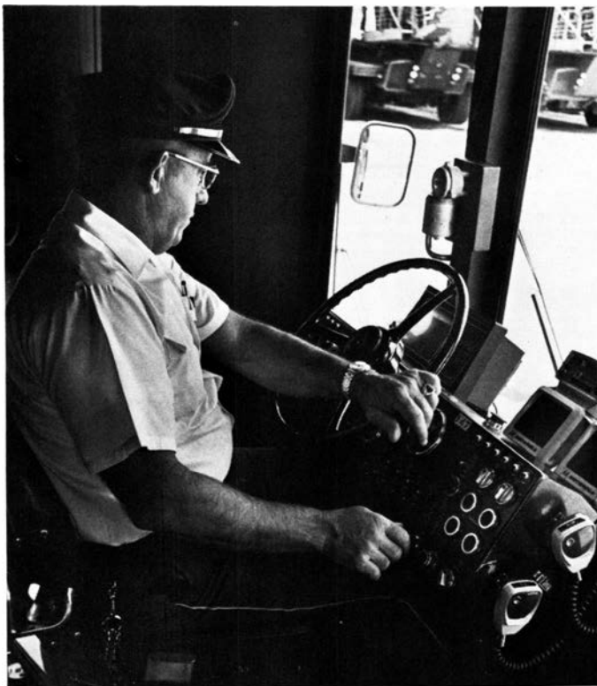
Burgess backs a Plane-Mate away from the terminal, using mirrors and a small television monitor that shows the roadway behind. The conventional lounge is double-ended.
