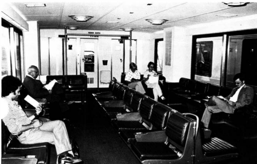
Passengers start to gather in a mobile lounge after the first call, relaxing in air conditioned comfort. There are 72 seats, with standing room for 28 more plus carry-on luggage.
