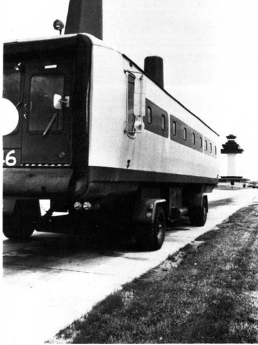
At left, the newer Plane-Mate lounge is parked near the maintenance area at Dulles. The protuberances atop it are the screw jacks on which the lounge raises and lowers itself. The transition device for the Plane-Mate (above) is a completely enclosed, full-width walkway that can be angled to mate with all jetliners, including the 747, L-1011 and DC-10.
