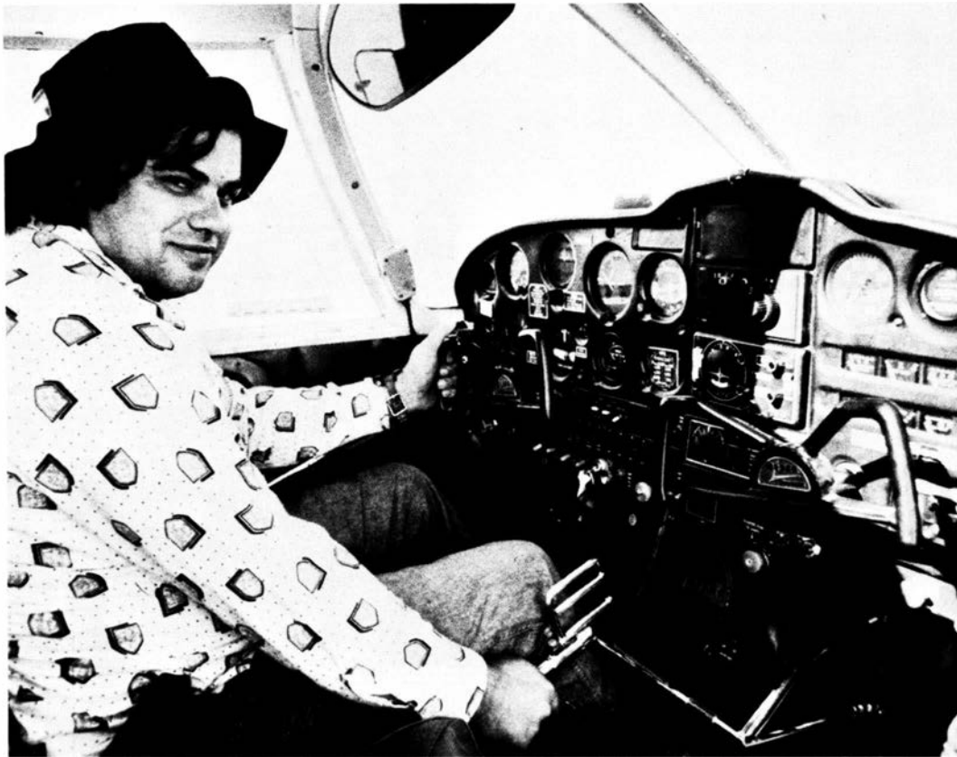
Going for his first solo, paraplegic veteran John McSwain demonstrates the hand control that operates the rudder and provides ground steering.
