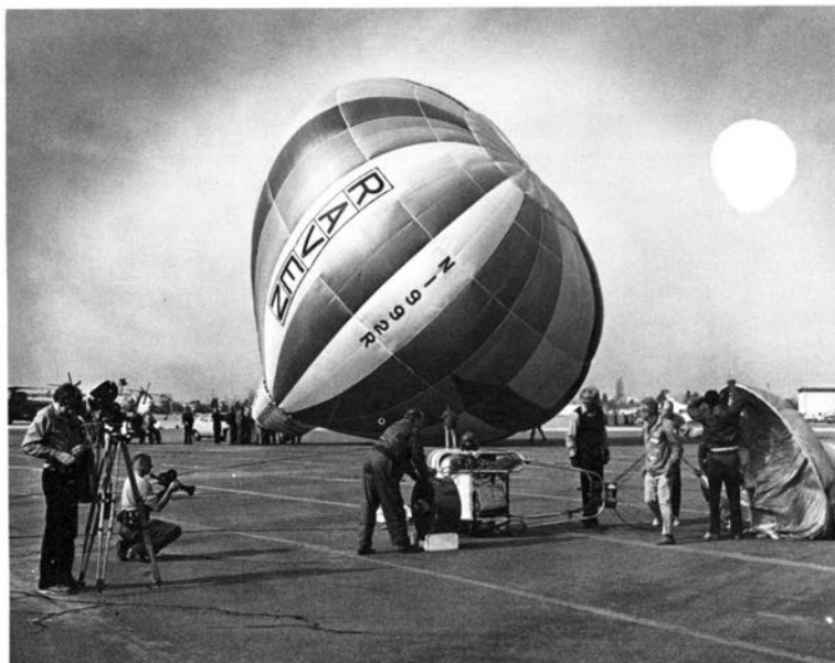
Camera crews record the preparations to inflate a balloon. At center, a man leans on a portable fan used to start the inflation before the propane burners are turned on.
