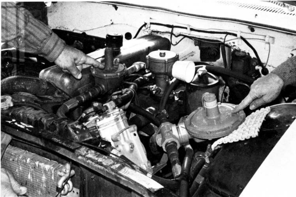
Under the hood of Goldsberry's converted gasoline-eater are indicated two of the three step-down regulators that supply the natural gas at very low pressures to the special-design carburetor shown at center.
