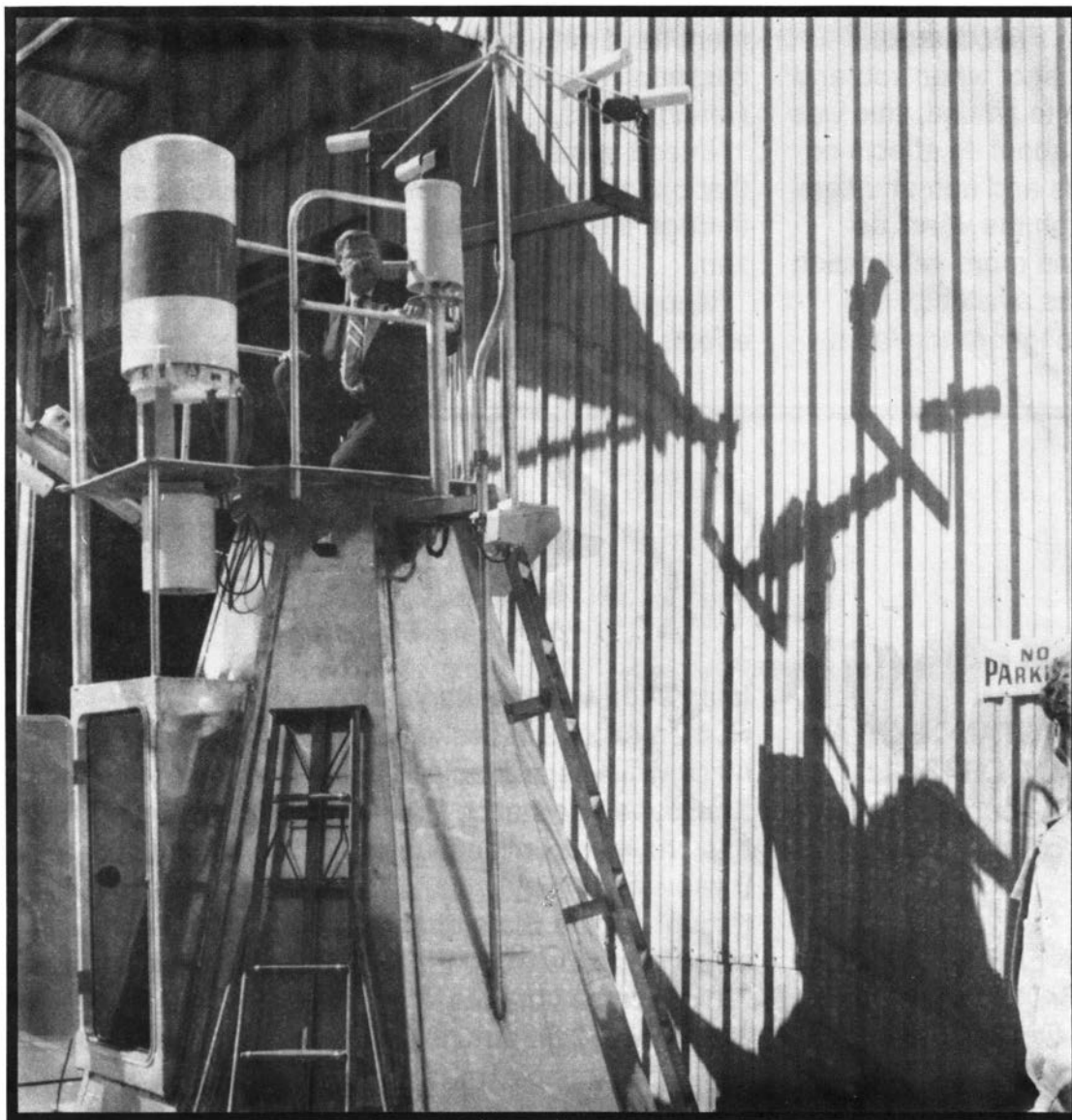
Robie Strickland , Airway Facilities Division Manager, checks out the equipment atop the AWOS tepee.
