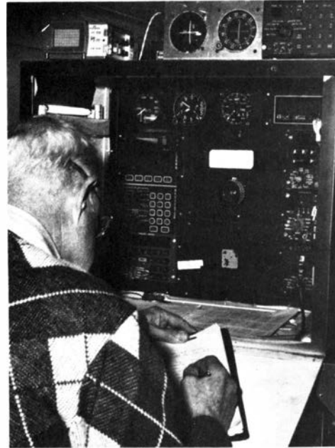
Arthur Heavener sets up LORAN-C and Omega photo panel displays prior to data flight.
