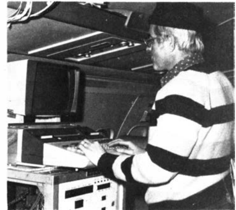
Thomas Wisser puts information on CRT display as the flight progresses. This display and auxiliary equipment tapes the INS, Omega, Loran C and other systems for later computer analysis.
